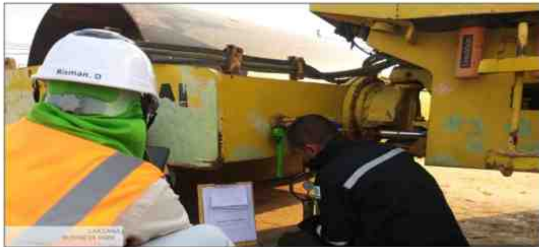
Gambar 4.9 Test California Bearing Ratio Lapangan (Test CBR)
