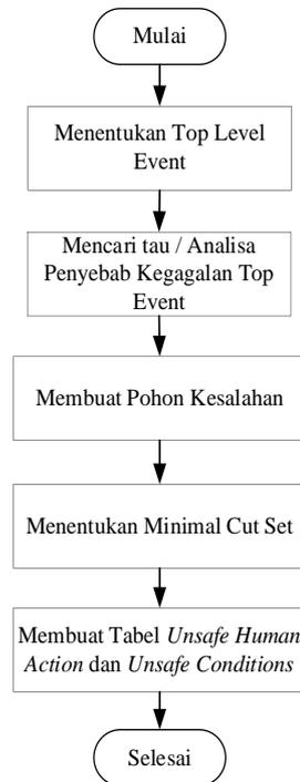
Gambar 3. 3 *Flowchart* Pengolahan Data *Fault Tree Analysis*
