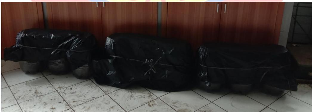
**Gambar 1.2** Perendaman Beton Yang Ditutupi Plastik
