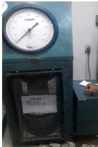
Gambar 3. 15 *Compressing Test Machine (CTM)*
