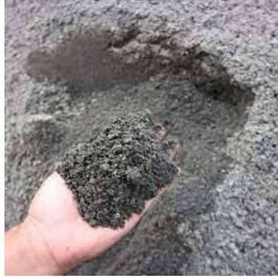
*Gambar 7.4 Agregat Halus Pasir*
