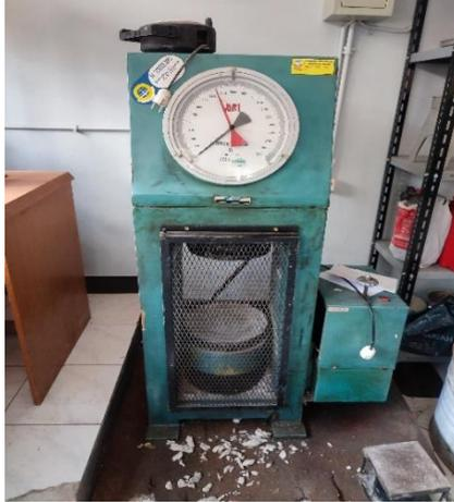
*Gambar 7.15 Compressing Test Machine*
