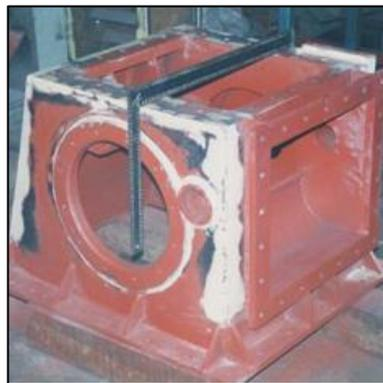
Gambar 2.17 Casing turbin
