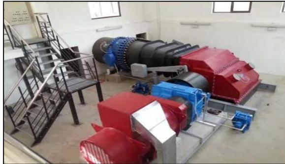
Gambar 2.7 Turbin *Cross-flow*
