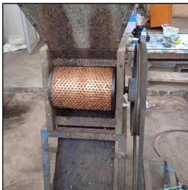
Gambar 2.54 MESIN PENGUPAS KULIT KOPI BASAH MPKK
