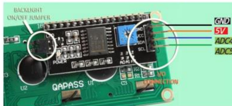
LCD display to Arduino wiring.
