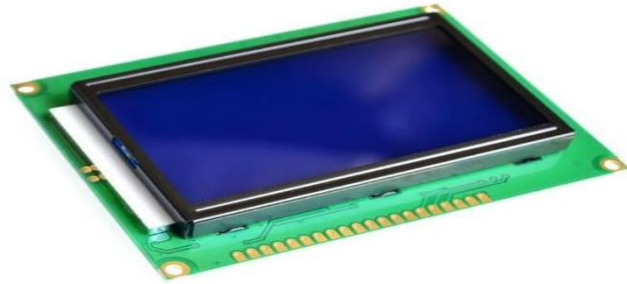
Gambar 2. 3 LCD ( Liquid Cristal Display ) 128 x 64
