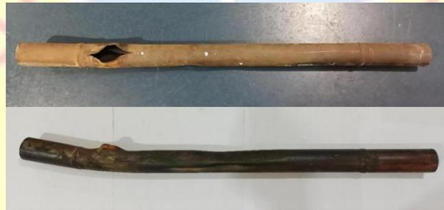
Gambar 4.1 Visual Sampel Tube Pecah
