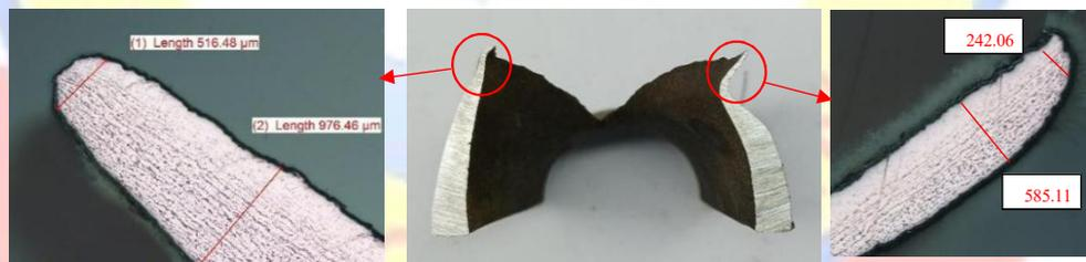
Gambar 4.7 Hasil Pengujian Thickness Area Pecah
