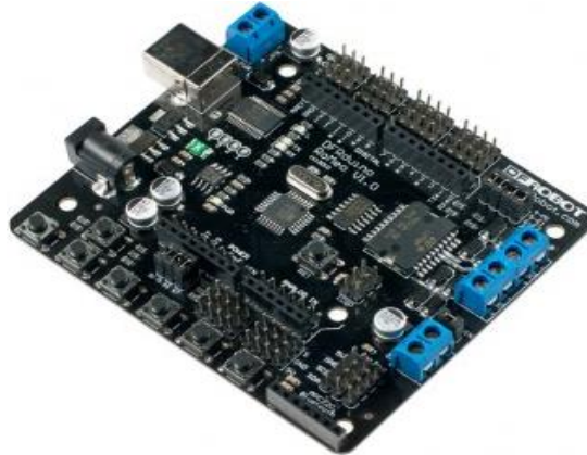
Gambar 13 Modul DFRobot Romeo All in One
