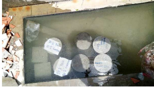
Gambar 4.7 Proses Perawatan Beton
