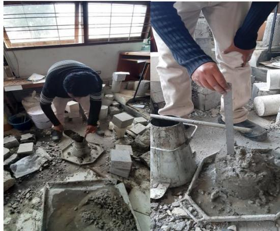
**Gambar 4.14.**Slump Test
