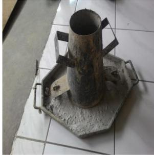
**Gambar 4.7.**Alat Slump
