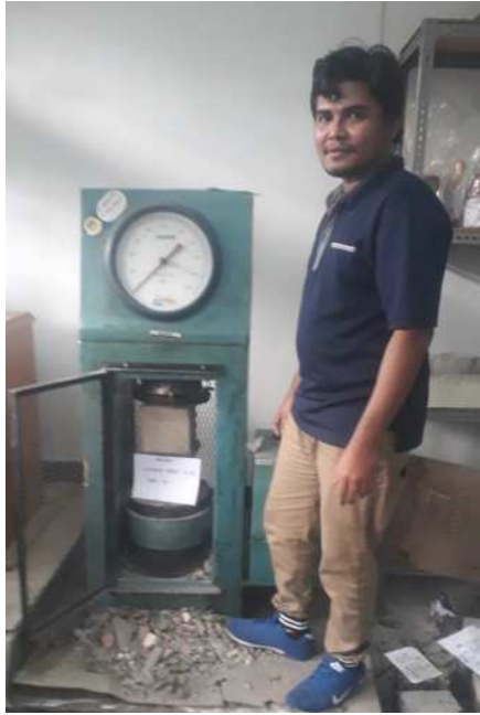
Gambar 4.6 Alat Uji Tekan ( Compression Testing Machine )
