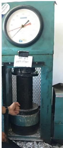
(Gambar 4.6. Pengujian benda uji kadar *fiberglass* 10%)
