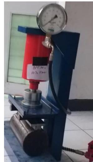
(Gambar 4.14. Pengujian benda uji 4 kadar *fiberglass* 10%)
