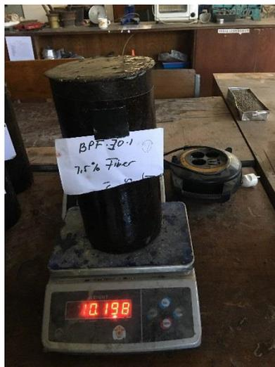
(Gambar 4.3. Benda uji 1 kadar *fiberglass* 7.5%)
