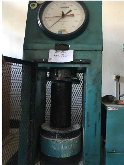
(Gambar 4.4. Pengujian benda uji kadar *fiberglass* 7.5%)
