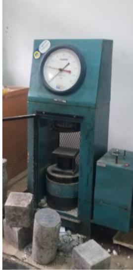
(Gambar 3.10. *Compressing test machine (CTM)*)
