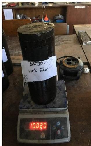
(Gambar 4.11. Benda uji 3 kadar fiberglass 7.5%)
