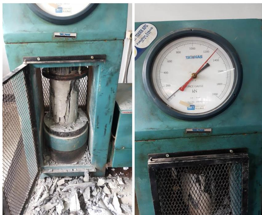
Gambar 4.9 Alat Compression Testing Machine
