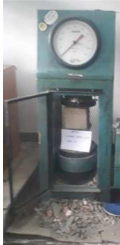
**Gambar 4.6** Alat Uji Tekan (*Compression Testing Machine*)
