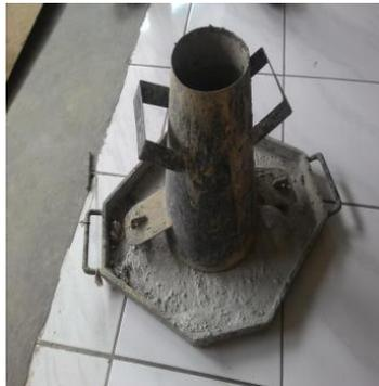
**Gambar 4.7** Alat Slump
