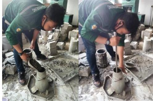
**Gambar 4.15** Slump Test
