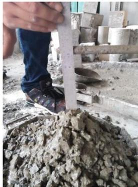
**Gambar 4.16** Hasil Slump Test
