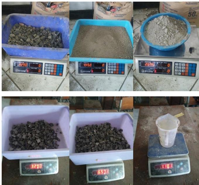
Gambar 4.12 Penimbangan Masing-Masing Material
