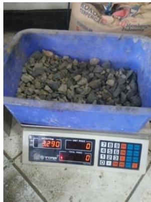
**Gambar 4.5** Proses Penimbangan Agregat
