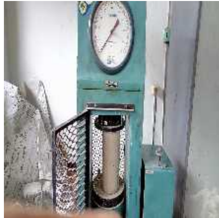
Gambar 4.9 Alat Compression Testing Machine
