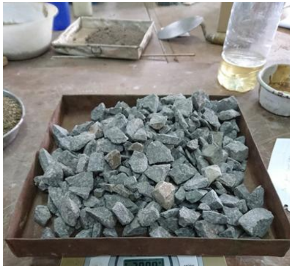
Gambar 13. Proses Pengujian Kadar Lumpur Agregat Kasar
