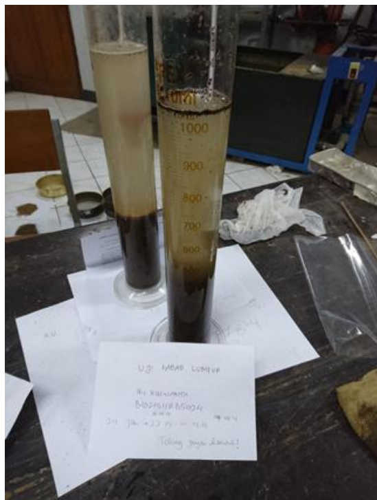
Gambar 9. Proses Pengujian Kadar Lumpur Agregat Halus
